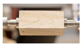
2. Turn the blank to the profile of your choice, down to the diameter of the bushings.
